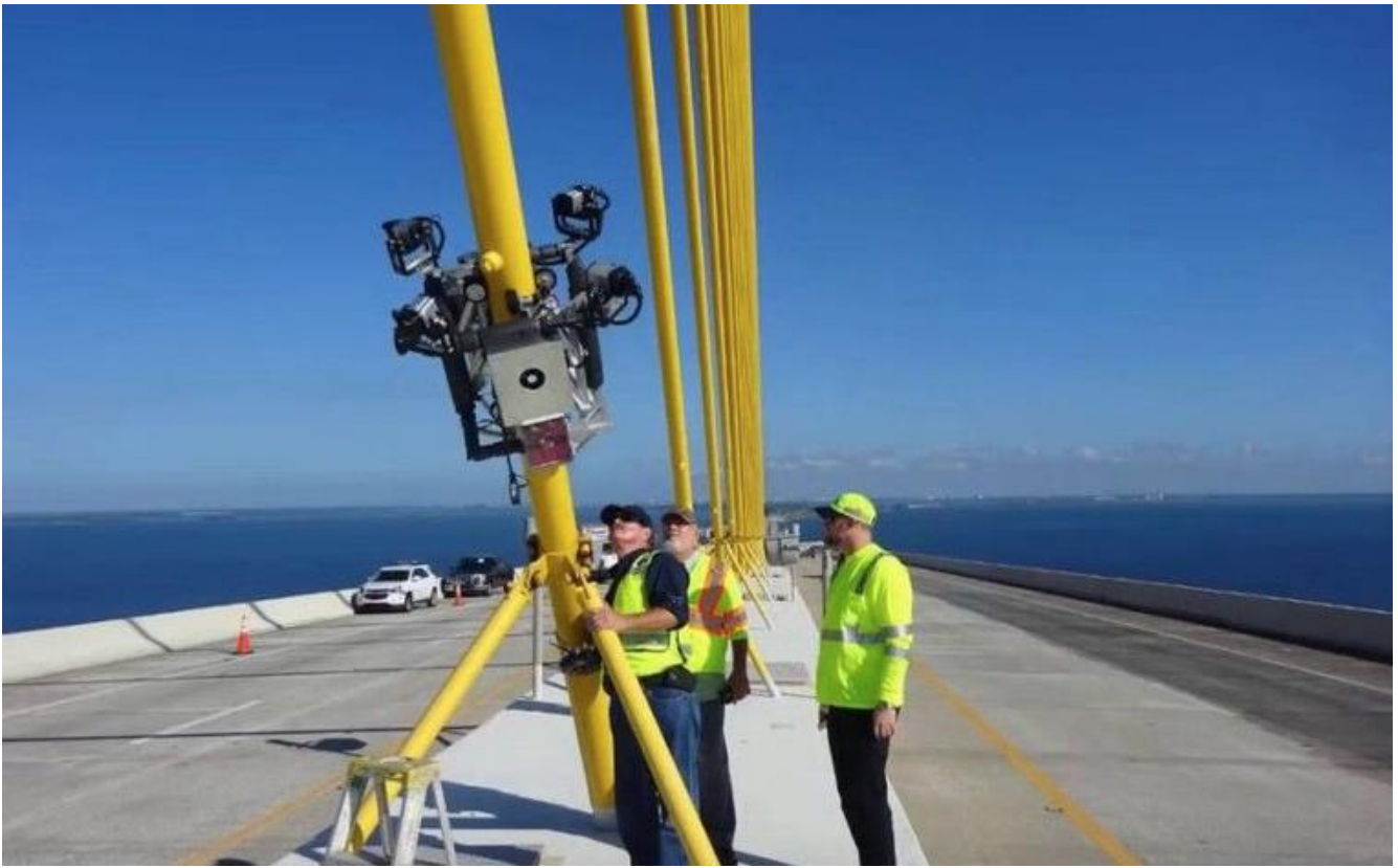
Infraspect manufactures road and bridge-scanning robotic technology (shown here).
